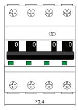
Construction of 4-pole width compared to traditional configuration offers space savings of up to 30%.
